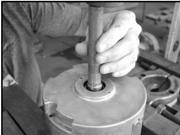
Figure 16b-8 Armature Removal
